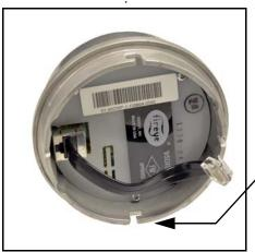
4. The displays for the InSight II are slotted in four (4) places to mate up with the key on the scanner and hold the display in position when the locking ring is removed..
