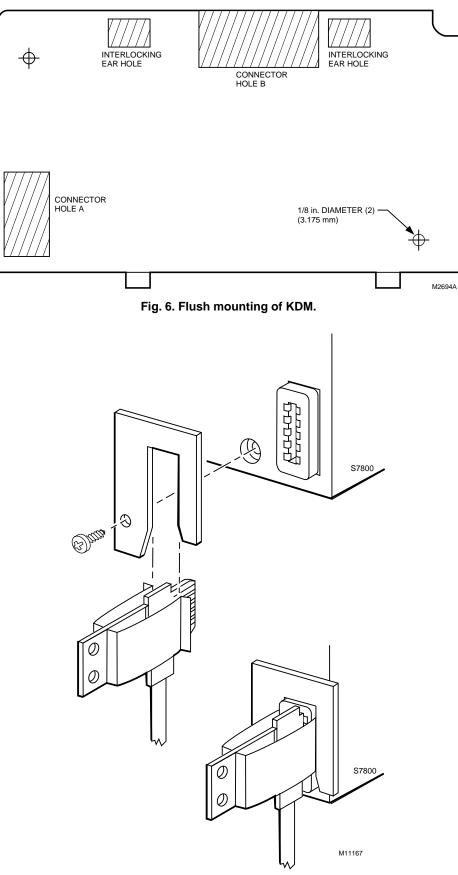
Fig. 7. Mounting 208702 Retainer Bracket.
