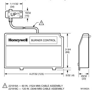
Fig. 1. Connector cover, connector dimensions, and cable length in in. (mm).
