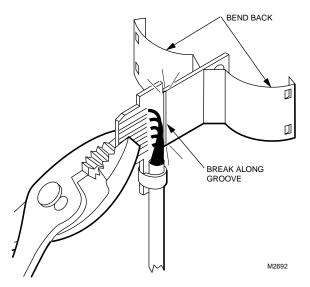
Fig. 5. Modified connector for bracket mounting.
