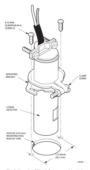
Fig. 8. Mounting C7044A Detector on blast tube.
