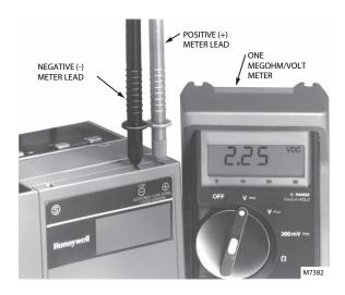
Fig. 11. Measuring flame signal voltage of 7800 SERIES controls.
