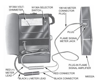
Fig. 10. Measuring microamp flame signal.
