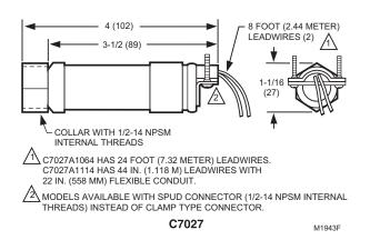
Fig. 1. Installation dimensions of C7027A in in. (mm).
