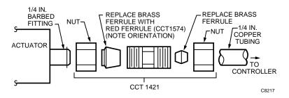
Fig. 10. Transition Piping for 1/4-Inch Barbed Fitting to 1/4-Inch Copper Tubing.
