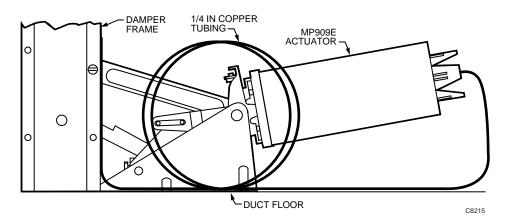
Fig. 11. Routing Copper Tubing Near Trunnion Pivot.
