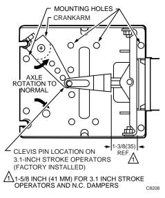
Fig. 3. External Installation.
