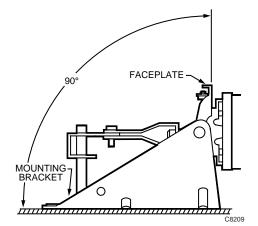
Fig. 2. External Mounting Faceplate Positioning.
