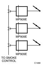
Fig. 12. MP909E Parallel Installation.
