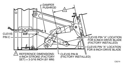
Fig. 8. Internal Mounting Normally Open Installation.
