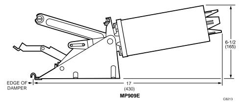
Fig. 7. Internal Mounting Normally Open Dimensions in Inches (Millimeters).
