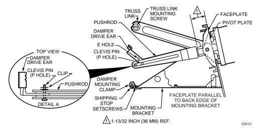
Fig. 6. Internal Mounting Normally Closed Damper.
