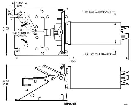
Fig 1. External Mounting Dimensions in Inches (Millimeters).
