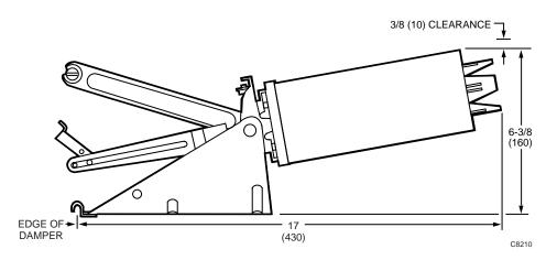
Fig. 5. Internally Mounted Normally Closed Mounting Dimensions in Inches (Millimeters).
