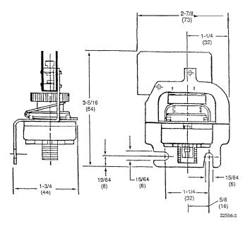
Fig. 3. P658E Switch Approximate Mounting Dimensions in Inches (Millimeters).
