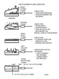
Fig. 6. Check burner flame condition.
