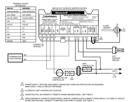
Fig. 5. Typical hookup when S8910U replaces Honeywell S89/S890.
