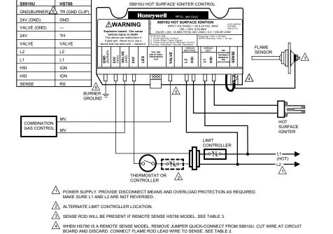
Use green ground adapter (supplied) to connect \$89100 gnd (Burner) to appliance chassis.
