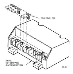
Fig. 2. Separating and installing selection tab.
