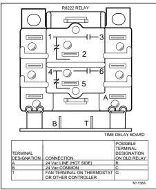
Fig. 2—ST82 circuit and terminal designations.
