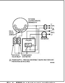
Fig. 4—ST82 in a heat pump application.
