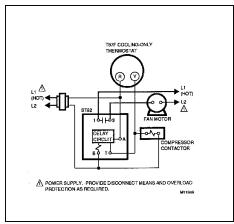
Fig. 3—ST82 in a cooling-only application.
