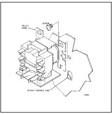
Fig. 1—Mounting relay on panel with shear-formed tab and one screw.
