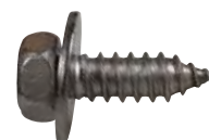
Universal Art. No. 140.7150/140.7150.BK P. Qty. 100/500 PH indented hex/washer screw, M6.3 x 19mm 18.8 SS
