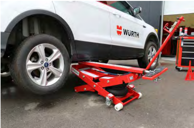
Lateral lifting with lift pad in use (included with Art. No. 995.110ML )
