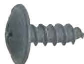
Nissan Art. No. 140.7075 - P. Qty. 100 Black Phosphate, PH truss head screw M4.8 - 1.61 x 15mm (#10 x 19/32) 14mm (9/16) Head O.D.
