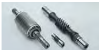
Bearing seats, repaired and then reworked
