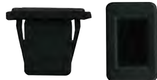
Rear Light Housing Upper Grommet Art. No. 502.20529 OEM #: 15745991
