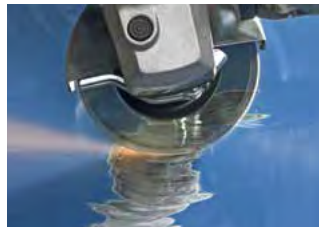
Grinding with Zebra slotted see-through disc: good view of the material being processed.
