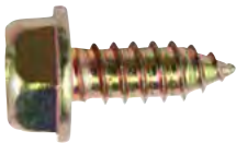
Universal Art. No. 140.17980 - P. Qty. 50 Yellow Zinc Plated, M6-1.81 x 16mm (1/4-14 x 5/8"), PH Hex Washer Head. 13mm (1/2") washer head O.D. 10mm Hex
