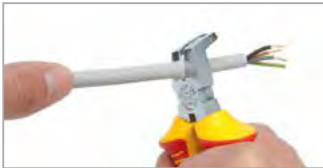
Cut cable with the side cutter
