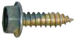
Honda, Geo Prism, Toyota Art. No. 140.7040/140.7040.BK P. Qty. 100/250 Yellow zinc, PH hex washer head screw M6 - 1.81 x 20mm (1/4" x 3/4") 12mm washer head O.D. 10mm Hex Honda 1990 - on
